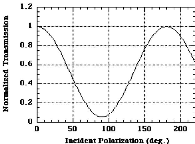
**Fig. 4** Normalized transmission of a micropolarizer element versus the incident polarization angle with respect to the polarizer polarization axis. The transmission extinction ratio is about 20.
