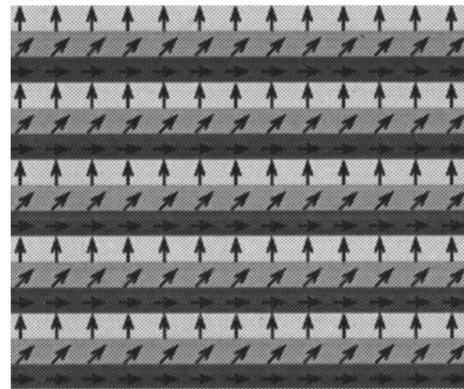
**Fig. 5** Polarization pattern of the three-state micropolarizer arrays.
