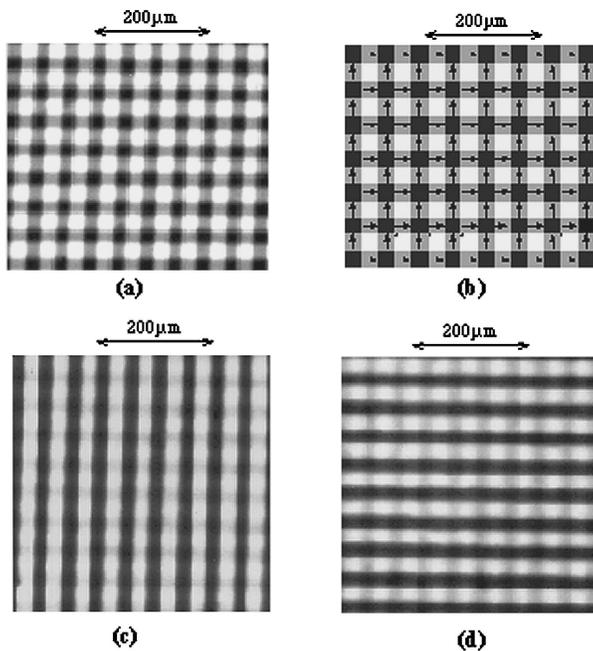
**Fig. 3** (a) Transmission photograph of the crossed micropolarizer arrays under unpolarized illumination, each polarizing element is  $25 \times 25 \mu\text{m}$ ; (b) Polarization orientation pattern in the micropolarizer arrays; (c) transmission photograph under horizontally polarized illumination; and (d) transmission photograph under vertically polarized illumination.
