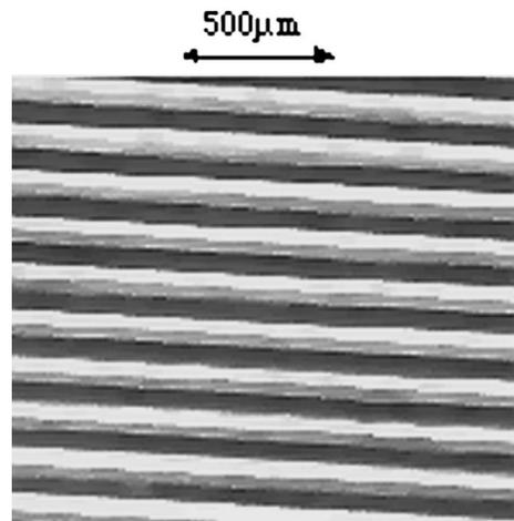
**Fig. 6** Photograph of the three-state (0, 45, 90 deg) micropolarizer scan lines. The width of each state is  $48 \mu\text{m}$ . The photograph was taken with linear polarized light in one polarization direction.
