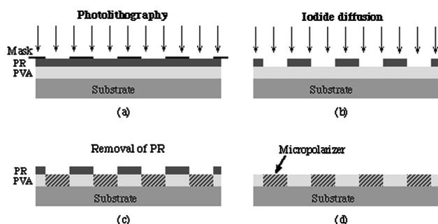
**Fig. 1** Fabrication of one layer of a PVA film micropolarizer: PR; photoresist.
