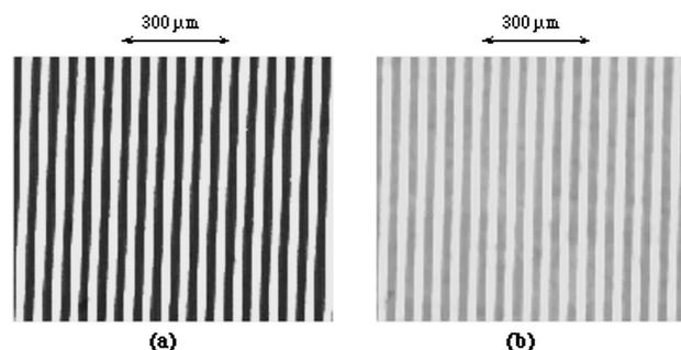
**Fig. 2** Transmission photographs of the micropolarizer strips. The width of each strip is  $25\ \mu\text{m}$ . (a) The illuminating light is polarized (a) orthogonally and (b) parallel to the micropolarizer polarization orientation.
