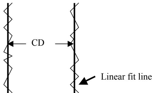
**Figure 2. The roughness is the deviation between individual edge locations and a fitted line.**
