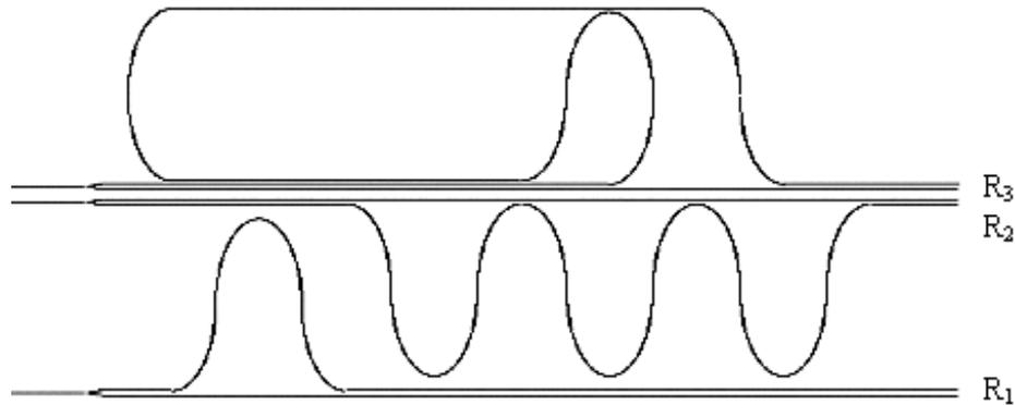
Figure 3 . PLC's for waveguide linear loss and curvature loss measurements.
