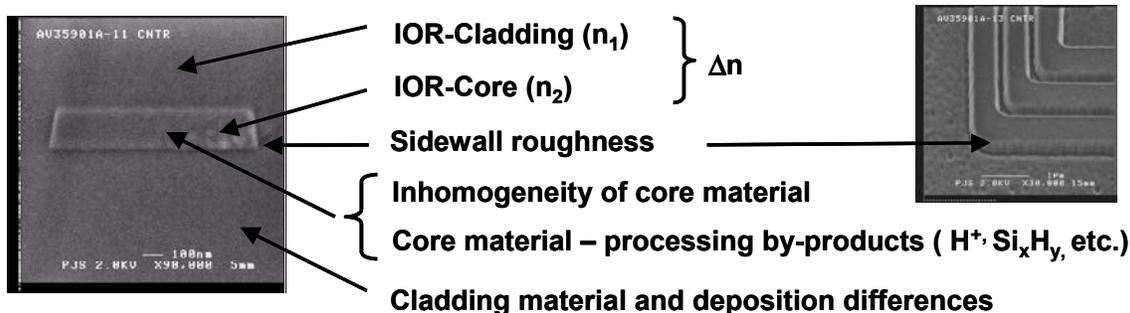
**Figure 1. Major issues impacting loss mechanisms in the  $\text{Si}_3\text{N}_4/\text{SiO}_2$  waveguide material system.**
