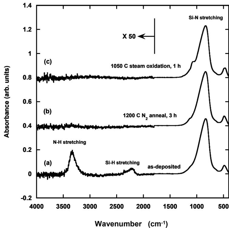
Figure 6, curves (a), (b) and (c). FTIR scan of  $\text{Si}_3\text{N}_4$  blanket film as deposited, annealed at 1200 degrees for 3 hrs., and 3 hr. 1200 °C anneal - followed by steam anneal at 1050 degree C for 1 hr. (a) As deposited  $\text{Si}_3\text{N}_4$  film showing N-H and Si-H stretching. (b) After 1200 °C anneal the peaks are vacant. (c) 3 hr. 1200 °C anneal followed by 1050 °C steam oxidation for 1 hr.
