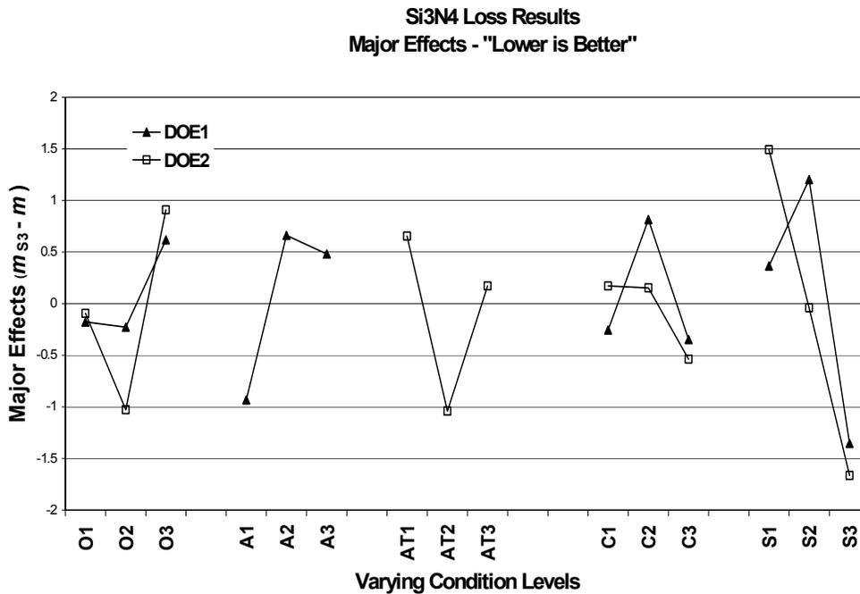
Figure 5. Waveguide loss results displayed as Major Effects calculated from Equation 2. DOE1 and DOE2 differ by the anneal experiment levels where An = anneal locations in the flow, and ATn = anneal duration time. Sidewall smoothing strategy 3, steam oxidation and HF strip show the biggest effect in reducing the linear loss.
