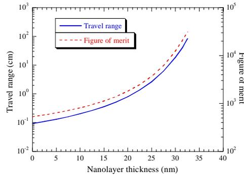
Fig. 3. The travel range and the figure of merit versus the thickness of nanolayers.
