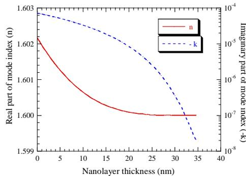
Fig. 2. The real part (solid line) and imaginary part (dashed line) of the mode index versus the nanolayer thickness.
