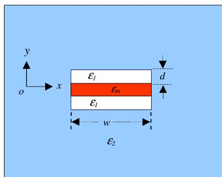
Fig. 1. The cross section of the finite width metal strip plasmon waveguide with dielectric nanolayers. The metal strip (red in the center) is sandwiched between two dielectric nanolayers of dielectric constant ( $\epsilon_1$ ) less than that of the dielectric cladding ( $\epsilon_2$ ).
