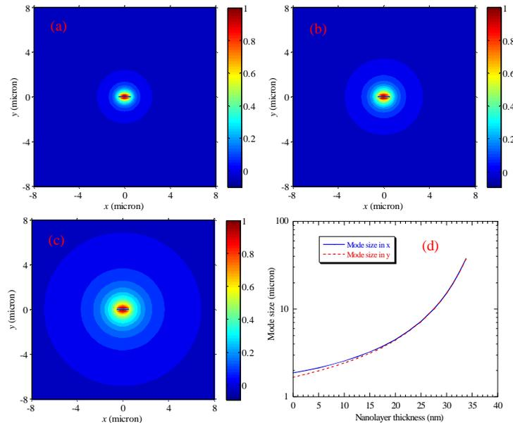
Fig. 4. The 2D power intensity plots of the symmetric plasmon modes without nanolayers (a)  $d = 0$  nm and with nanolayers of thickness (b)  $d = 10$  nm and (c)  $d = 20$  nm; the (d) shows the mode spatial extents in the x and y directions versus the nanolayer thickness.
